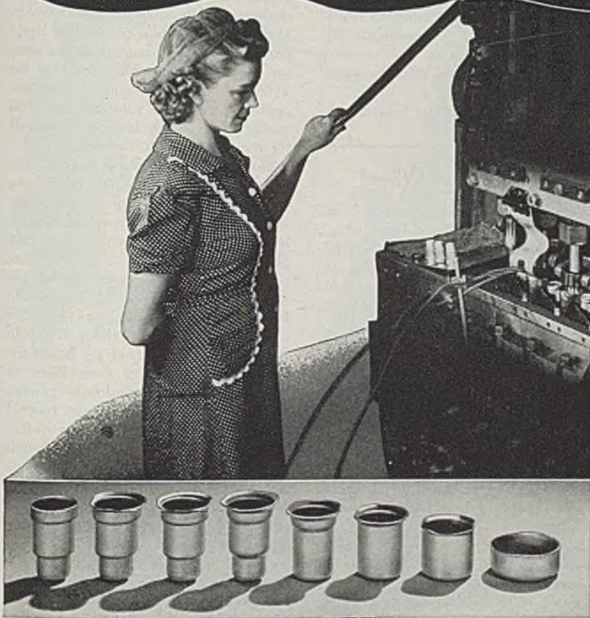
Sockets are formed on a 9-plunger press from cold rolled steel, .034" thick. Stock is pre-zinc coated; coating acts as a lubricant and helps insure a final finish which will require little or no buffing or polishing.
