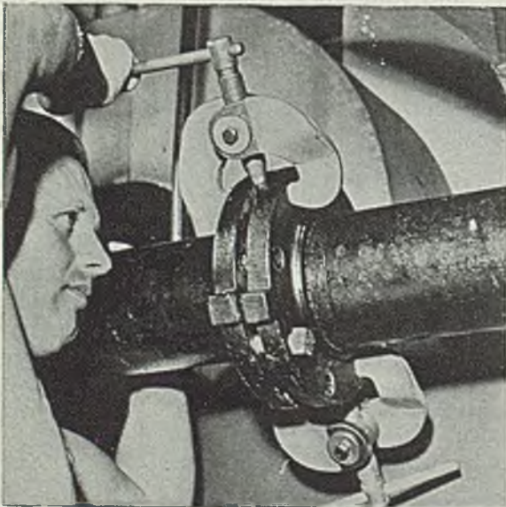
PIPE FLANGE OPENER: Job of opening pipe flanges for removing gaskets is speeded, simplified by these Flange-Jacks made by T. G. Persson Co., 224 Glenwood avenue, Bloomfield, N. J. Jacks are capable of opening joints against a load of 15 tons without damage to flanges. As pressure is exerted, flanges open evenly, without shock and in continuous alignment. Closures are accomplished in similar manner. Jaws are heavy one-piece steel forgings with case-hardened screw points
