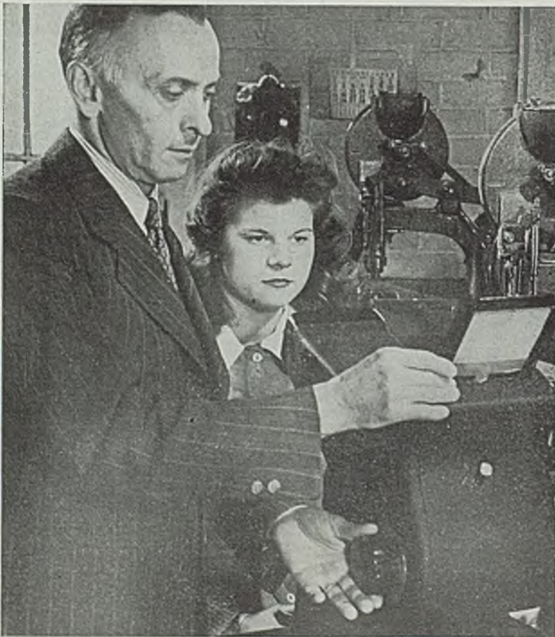
CHECKING INDUSTRIAL VISION: Detection of visually unfit employees needing eye examination and correction is possible in three or four minutes through a newly developed, portable sight-screener instrument announced by the American Optical Co., Southbridge, Mass. Data on 14 different visual functions can be obtained through the instrument, facilitating promotion of industrial efficiency and safety
