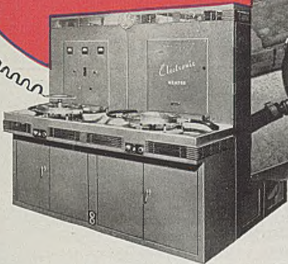
▲ G-E 50 kw electronic heater, used at Studebaker's South Bend plant
