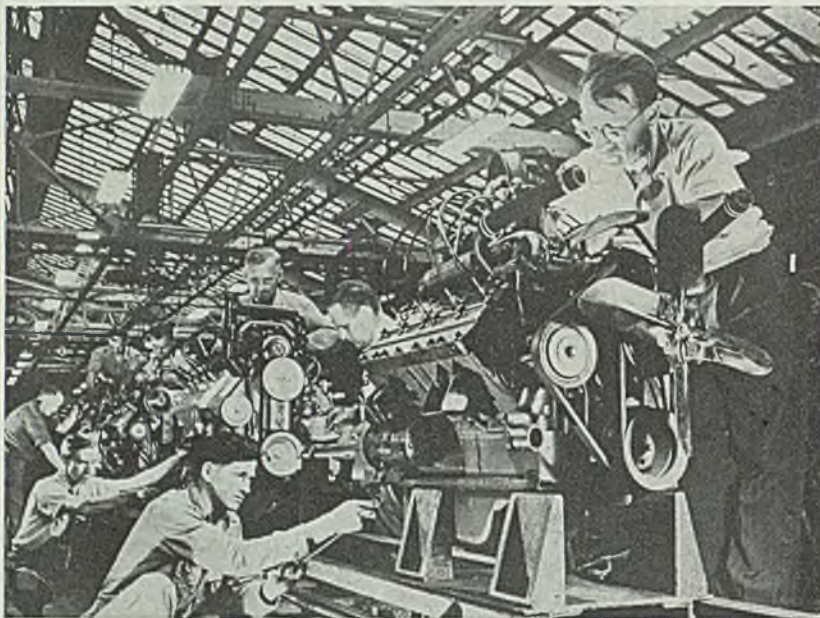
BACK TO PEACE: Engines on the assembly line of the Cadillac Division of General Motors in Detroit. During the war these engines, adapted to war needs, powered Cadillac-built light tanks
