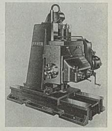
machine. For large boring or facing operations and back facing of flanges, a face plate with tool block slide may be mounted on head of work spindle.
