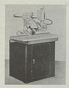
chinery, manufactured by American Saw Mill Machinery Co., Hackettstown, N. J. Made principally of light, nonrusting magnesium, the unit complete with carrying frame and 11/2 hp electric motor weighs approximately 200 lbs. It has a 3 x 16 in. crosscut and 201/2-in wide ripping capacity. Attachments may be installed for notching, routing, shaping, dadoing, sanding, boring and other jobs found in the pattern shop.
