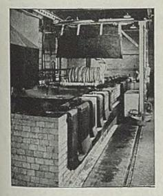
CLEANING AND COATING — RB&W draws its own wire to assure close tolerances vital to perfect cold-heading. Pickling — in this scientifically controlled cleaning department — leaves the wire free from mill scale, and provides opportunity to coat it properly for subsequent drawing and heading.
