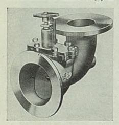
Zurn Mfg. Co., Erie, Pa. Units feature a swing check flap suspended from a full floating pin fulcrum to insure positive full surface contact between ground face of flap and seat to eliminate fouling. Flap can be removed and replaced.
