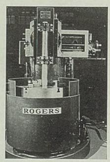
cult boring operations. The heavy bar arrangement and 3-jaw combination chuck il'ustrated, are for single-operation work not requiring turret.
