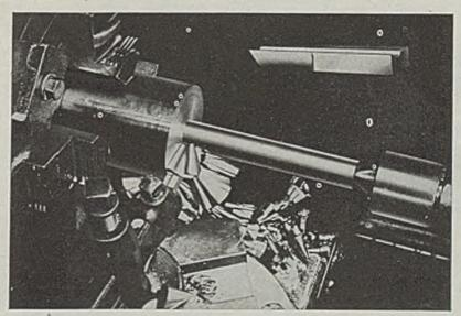
TRUE molecular cleavage and a shearcutting action in the machining of metals is achieved by a tool bit developed by Fearless Tool Co. The Los Angeles concern reports the faster cutting speeds and lack of heat usually generated by such cutting action reduces production time as much as 50 per cent. It also is said to lower power consumption 70 per cent, reduce regrinding operations more than 50 per cent, and increase tool life
