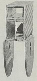
Gun Mount Part: Fabricated by brazing steel sprocket to heavy steel tube. Ring of 3/64-in. alloy is preplaced above sprocket, followed by fast induction heating. Penetration is complete
