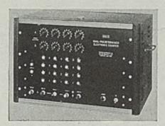
which any number from 0 to 10,000 may be initially setup by rotary switches mounted on front panel, Power for operation is obtained from a 110 v 60 cycle circuit.
