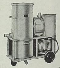
unit more compact, length, width, height and weight have been reduced. Motor mounting is reversed from above vacuum producer, eliminating two castings and putting vacuum produced directly in line with dust tank.
