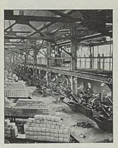
NUT FITTING AND PACKING—Fitting nut to bolt is a final inspection of the product, and provides protection for the threads during shipping and handling. From these automatic machines, assembled bolts and nuts are put into durable cartons and packages labeled for maximum visibility.
