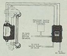
Probe fitting is mounted parallel to the water column and wired to the control. Current required is 115-230 v, 60 cycles ac.
