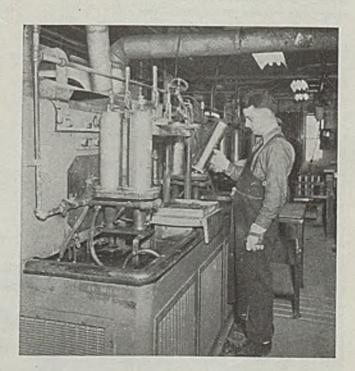
Setup for Induction Brazing: Shell bases and bodies are heated two at a time in this Tocco induction heating machine while another two-unit station is loaded. Clamps on top of shell apply just enough pressure to insure base settling accurately in place when brazing alloy melts and flows. Note ventilating facilities for removing fumes. Brazing time 49 sec per shell
