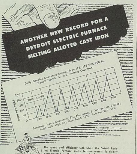
demonstrated in the above graph of a typical day's operation. In 814 hours, a Type LFY, 175 Kw, 700 lb.
