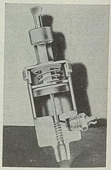
dispense oil or grease in a measured, uniform flow to moving bearings, and stop when bearing becomes motionless. Offered in four sizes, the pressure-filled units have lubricating capacities ranging from ½ to 8 oz. Six interchangeable valves exert varying degrees of feed on greases of different densities. Steel 6/10/46; Item No. 9267
