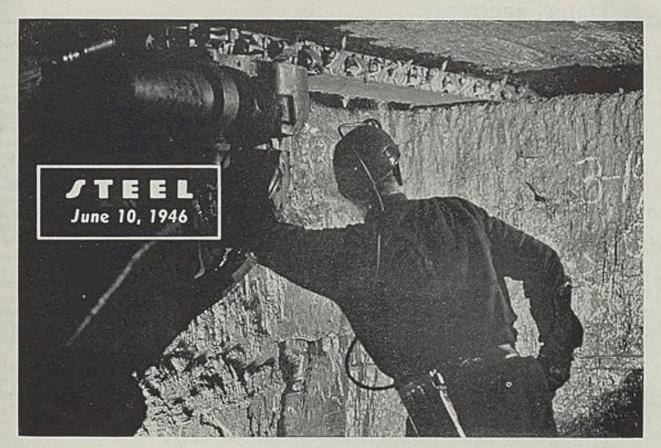
Mechanized coal mining is expected to be further emphasized by the increased costs of labor resulting from the recent coal wage settlement. This photo shows a universal cutting machine which slices nine feet deep in the Leisenring No. 2 mine of the II. C. Frick Coke Co. near Uniontown, Pa.
