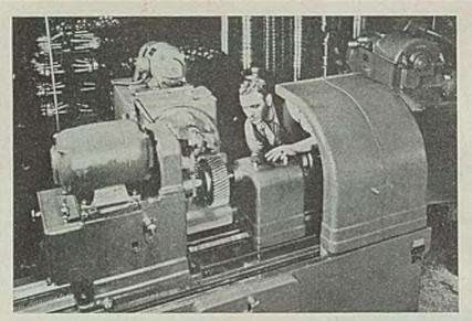
VERSATILE GEAR FINISHER: Gears up to 24 in. OD are handled by this Michigan Tool Co. rotary gear finisher which is making it possible to precision finish gears in job lots at the plant of Fairfield Mfg. Co., Lafayette, Ind. Machine finishes most of the spur and helical gears eventually going into tractors, buses and industrial machinery. Approximately 2500 different items are routed by the company over its production lines in a nomal year
