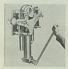
chine to move or shift pipe. Bending is as readily and easily performed as bends made to a lesser radii. Illustration shows bender completing a 180 degree bend. Steel 6/10/46; Item No. 9246
