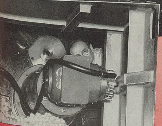
This right-angle boring head runs into deep wells and interiors for machining on surfaces like the side cushion guides on the press bed shown here. Complete internal milling at any angle is possible in one setup.
