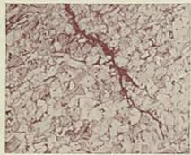
Photomicrograph of fatigue crack in silicon aluminum bronze developed in laboratory fatigue test after 10,000,000 cycles at a stress of 45,000 psi.
