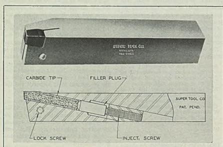
EJECTOR TYPE CARBIDE TOOL: This tool bit designed recently by Super Tool Co., Detroit, eliminates outside holding mechanism which frequently interferes with flow of chips. Tool consists of holder which is supplied in standard sizes, and an easily replaced mechanically-held insert bit of solid carbide. Bits are large and can be ejected easily for regrinding; angle at which they are set enables user to sharpen tool with minimum loss of carbide
