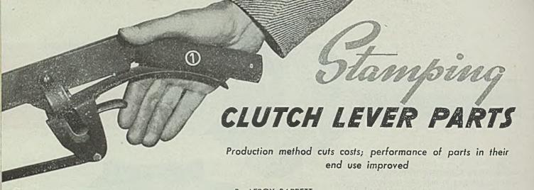
STAMPING of the two parts of a clutch lever has brought about an economy in material and production costs at the farm equipment division of Ellinwood Industries, Los Angeles. The new lever, shown in Fig. 1, was conceived by Anton Braun, research technician in the experimental and development department, and consisted of two steel stampings assembled with a steel pin that is staked after assembly.
