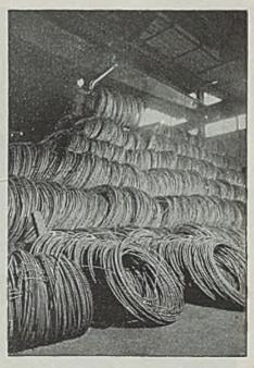
BOLTS BY BILLIONS — RB&W maintains stocks of raw material that are large enough to provide flexibility for a wide range of fastener production. This raw material is subject to careful analysis in RB&W's completely-equipped laboratory.
