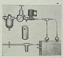
spray with its two or four nozzles and humidistat control. Nozzles can be set at various angles to increase efficiency of moisture distribution. Compressed air is utilized to produce an exceedingly fine, round spray. A complete 2-nozzle unit is illustrated.
