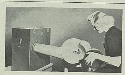
DUCTLESS DUST COLLECTING: Manufacturer of sports equipment solved dust problem on this buffing-finishing operation on leather goods by utilizing standard Dustkop dust collector made by Aget-Detroit Co., Ann Arbor, Mich., and hood and connecting pipe shown above. Installation is said to have been completed in a few minutes
