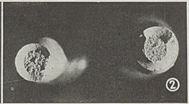
Fig. 2—Cup and cone fracture caused by introduction of radial principle stresses due to neck notch. Specimen at left 0.20 C steel, right 0.40 C steel
