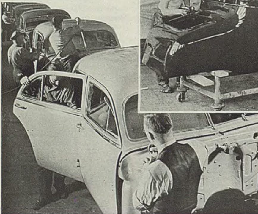
PROGRESS: More than a quarter of a century's progress is shown in these two pictures contrasting the same operation at a Fisher Body plant. Workmen, above, are touching up the varnish on a smart coupe of about 1920 vintage; on the left, a modern assembly line touch-up requires several painters and the inspector in the foreground
