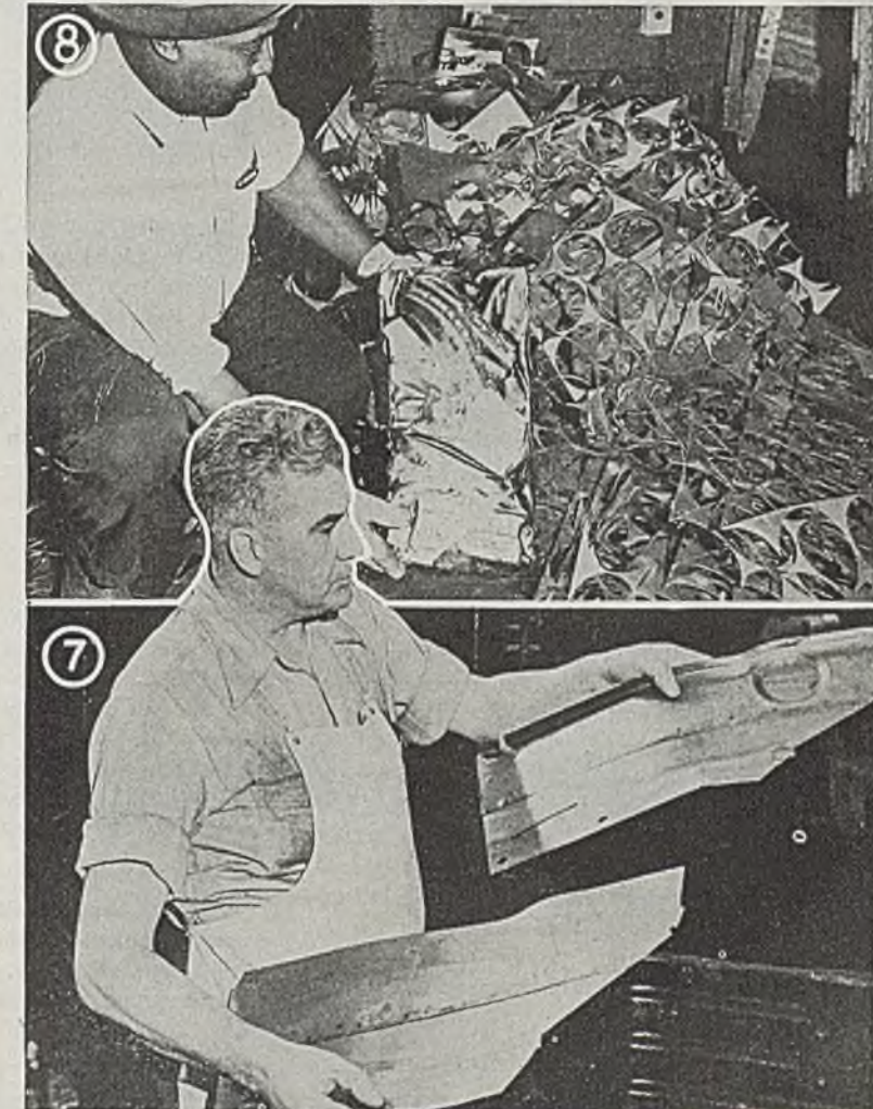
Fig. 5—After the deep drawing process that forms the rear fender, the four irregular flash pieces held by workers at left and right are trimmed from the edges and used to form other body parts
