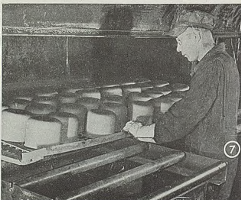
Fig. 7—Regulating covers on trays being withdrawn from the annealing furnace
