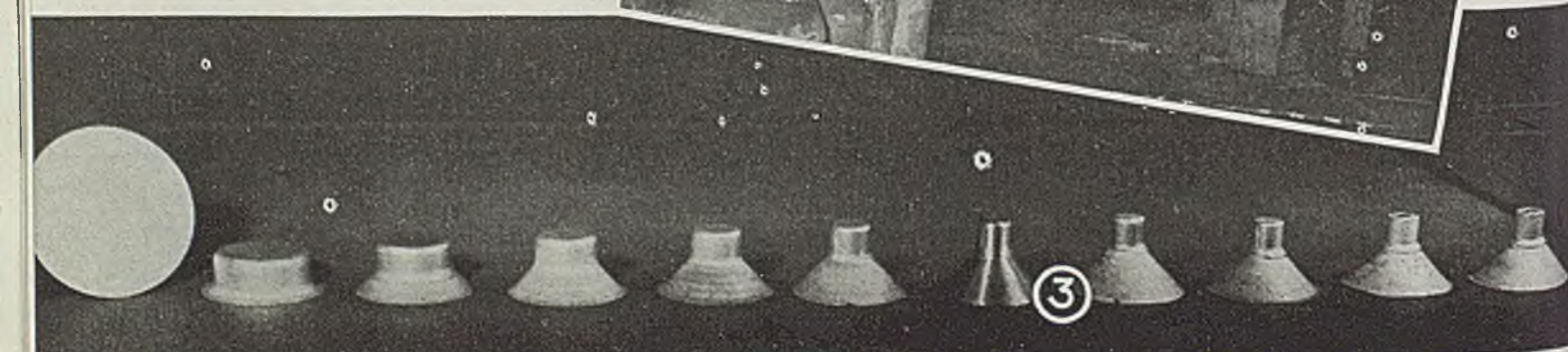
Fig. 2—McCormick-Deering 50-lb stainless steel milker pail after bulging in special HPM 750 ton press. Photos from International Harvester, by G. F. Zimmermann
