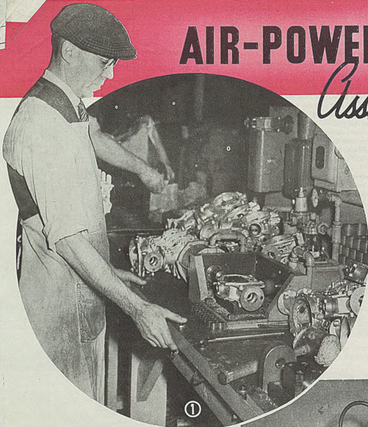
Fig. 1—Both hands must be used by operator to operate air pistons of this jig which presses two bushings into a wringer head
