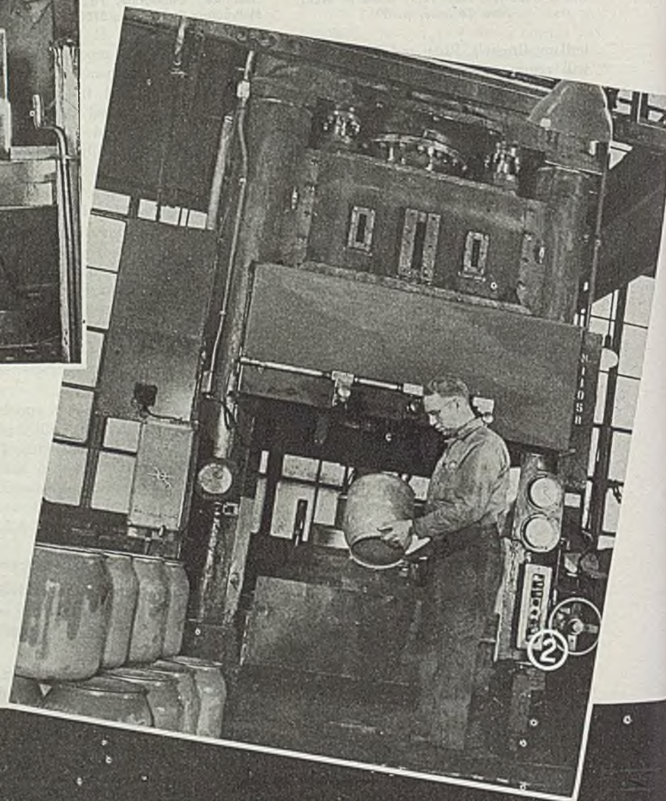
Fig. 1—Deep drawn shell to be formed into a 50-lb capacity milker pail has already gone through four draws, a form flange and a trim flange operation on this hydraulic press. Here it is being loaded onto the "bulging" dies where hydraulic fluid under 3000 psi will expand pail against die cavity to produce shape that is desired
