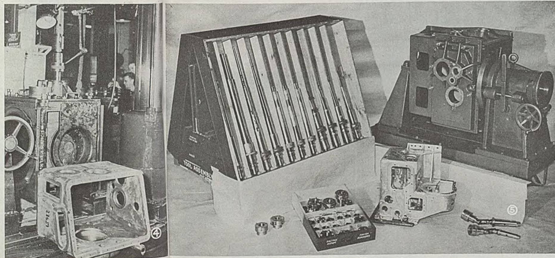
Fig. 4—Radial drill working frame shown in foreground in a single trunnion fixture. Note double universal joint for driving bars holding cutters. This prevents drill spindle from "crowding" the tools which are guided entirely by bushing in fixture. Thus, fixture alone determines accuracy of work, permitting exceptionally close tolerances
