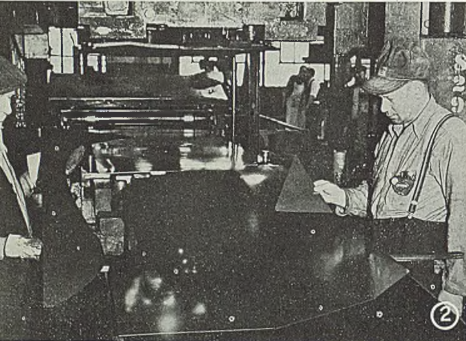
Fig. 2—All flat scrap pieces from fender blanks are saved and sorted to be drawn into smaller parts
