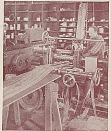
Fig. 2. Slitting machine, shearing metal into narrow strips.
