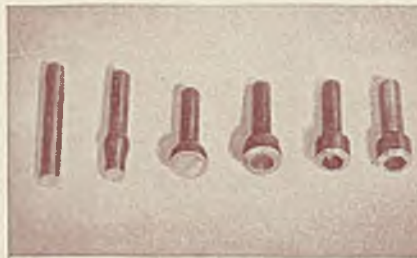
The photograph shows an Allen head bolt, made by cold heading Duronze V wire.
