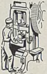
Plate samples are punched to rough form, then milled. Others are sawed, turned, drilled etc., as required.
