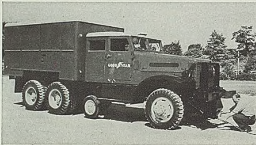
TESTS TIRES, WHEELS: This dynamometer truck, adapted by Goodyear Tire & Rubber Co., Akron, from a 6-wheel drive Army truck, is used to test large tires and wheel equipment for off-the-road vehicles and machinery. The free rolling wheel below the cab is used to measure distance and speed during testing operations
