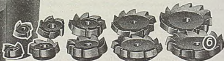
Fig. 6—Ring dies made from an oil-hardening tool steel which can be tempered to a rockwell C hardness of 65. These dies are made in sizes up to and including 16 in. outside diameter and in lengths up to 15 in.
