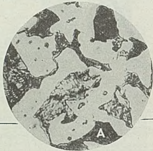
Fig. 1—Effect of structure upon properties. Diagrams and photomicrographs (1000X) are from 0.35 per cent carbon steel, 1/2-in. NC threads, extruded and roll threaded
