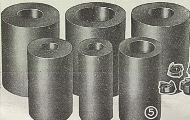
Fig. 5—Various size cutter bodies also made by the cast-to-shape technique. Steel used for these was of the high carbon-high chromium air-hardening type
