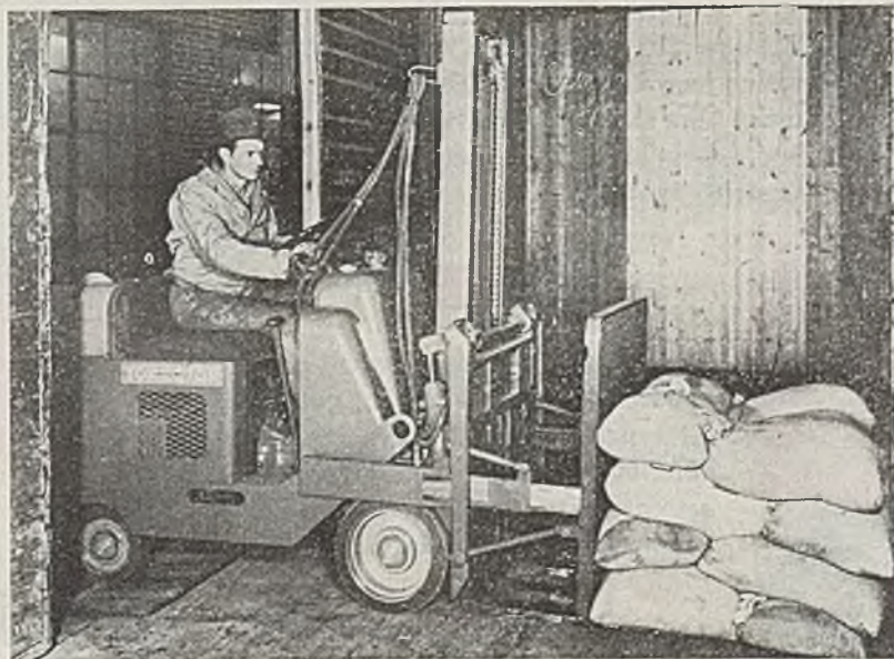
LIFT TRUCK UNLOADER: Shown here loading box car is new hydraulically operated device manufactured by Towmotor Corp., Cleveland, for use in unloading lift trucks. To push load off forks driver operates two double-acting cylinders, one on each side, moving vertical rack forward. Forty-ton box car is said to be loaded in 28½-min., reducing loading costs from 50 to 20 cents per ton. Pulling power of loader is equal to pushing power
