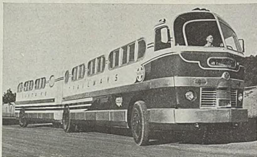
LUXURY BUS: This 60-foot articulated bus, featuring aluminum and magnesium, was built for Sante Fe Trail Transportation Co. by Permanente Metals Corp. It will be tested by the Sante Fe company and may be placed in regular service on the line
