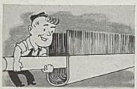
3 Next, a plated steel wire is laid along the channel on top of the filler material to anchor it permanently in position.
