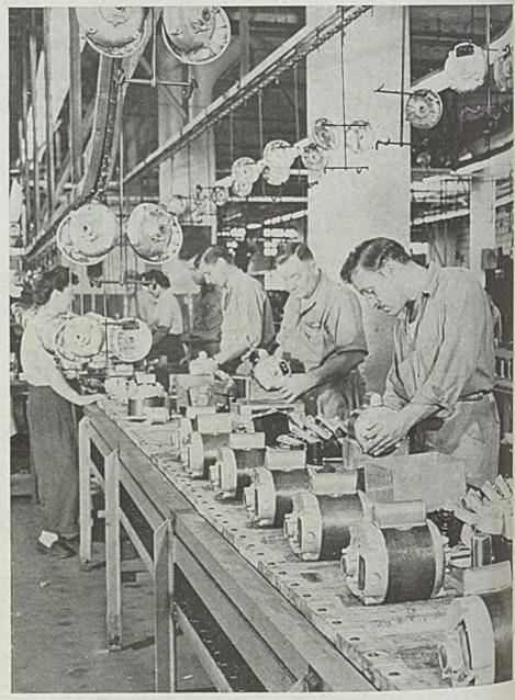
Fractional horsepower motors move down the final assembly line at Plant 7, Jack & Heintz Precision Industries Inc., Cleveland
