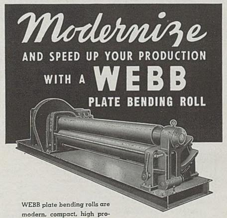
duction machines. Made in a complete range of sizes and capacities, these rolls are being used on high quantity production rolling in all types of metal shops throughout the United States. These rolls are made in both pyramid and pinch types.
