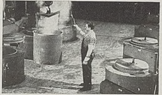
ANNEALING —In gas-fired batch-type draw furnaces, RB&W rivets are annealed to remove cold heading stresses and to assure proper hardness. These furnaces are accurately controlled to provide thorough and accurate heating.
