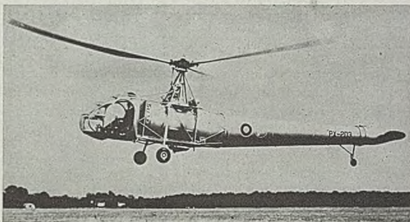
OFF SECRET LIST: This research helicopter, Cierva Weir-9, which had been on Britain's secret list, is shown in its first public demonstration at Southampton, England. The craft has jet torque reaction and directional control provided by a laterally directed jet squirting sideways of the tail. "Urge" for the jet is supplied by exhaust and the fan used to cool the plane's engine. NEA photo
