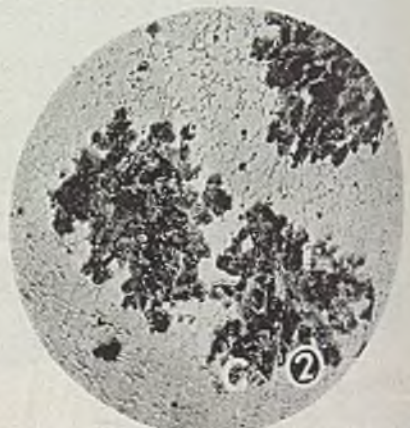
Fig. 2—Effect of structures of Fig. 1 on the stability of austenite at 1300° F. Sample of photomicrograph A was austenitized 15 min at 1400° F, that of B for 90 min, and that of C for 240 min. All specimens were then cooled to 1300° F, held 2 hours, water quenched. Any untransformed austenite would, on quenching, become martensite (light areas in photomicrograph B and C). Dark areas are pearlite. Picral etch.—Magnification 50X
