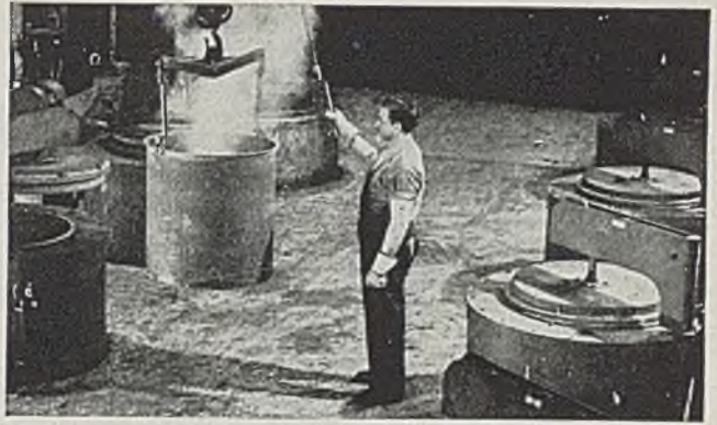
ANNEALING —In gas-fired batch-type draw furnaces, RB&W rivets are annealed to remove cold heading stresses and to assure proper hardness. These furnaces are accurately controlled to provide thorough and accurate heating.
