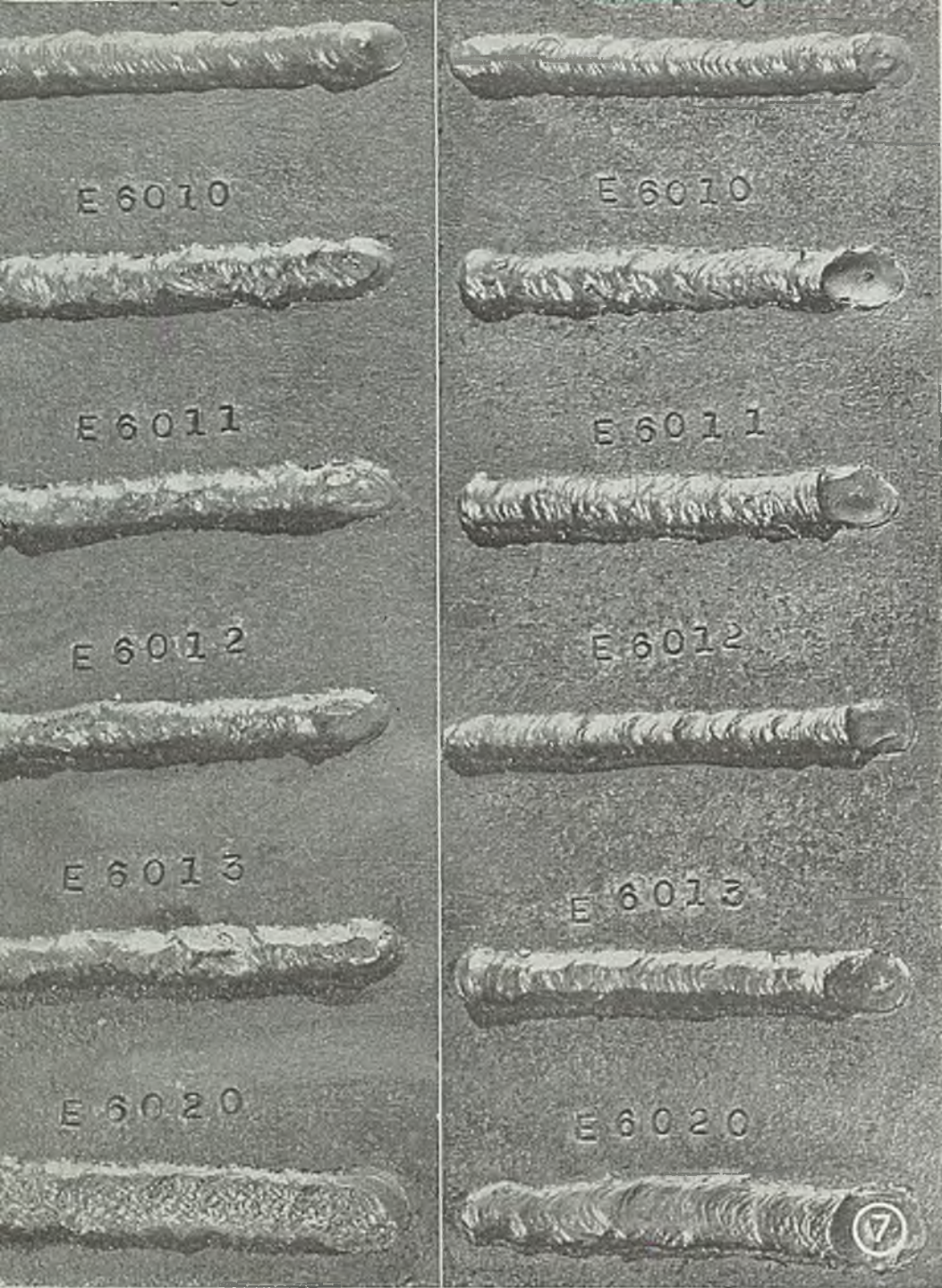
Fig. 7—Beads on high sulphur steel on left as compared with mill steel on right show that all welds except the lime-ferritic suffer from effects of sulphur
