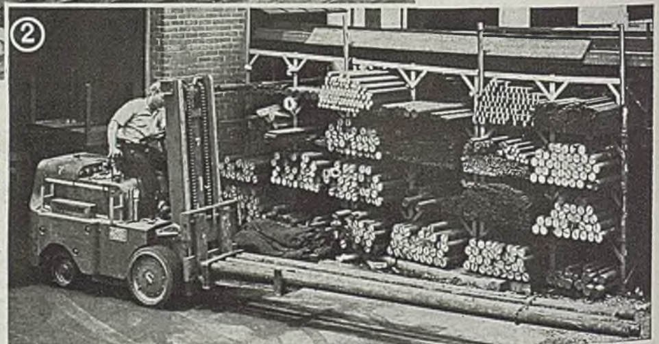
Fig. 2—Another view of rig in Fig. 3 showing heavy load of rounds in proper position ready for transporting
