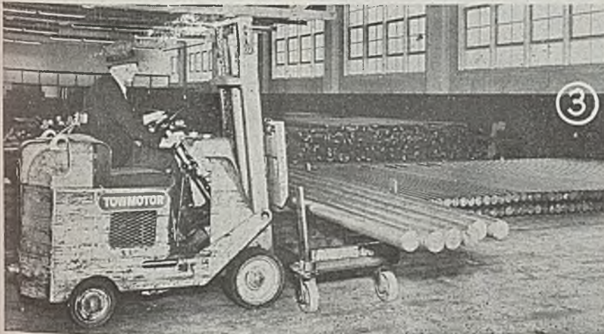
Fig. 3—This specially designed wagon has traverse boards so that forks of truck can slide under bars
