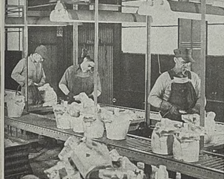
Fig. 5—Heads are spot-checked during forging operation. Here inspector is putting a cylinder head through caustic soda, nitric acid and hot water rinses preparatory to visual examination
