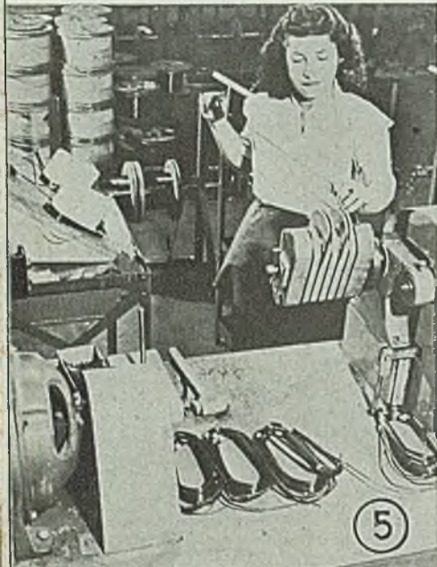
Fig. 5—Locating a crossover sleeve, one of new steps in procedure of winding coils of synthetic resin insulated copper wire
