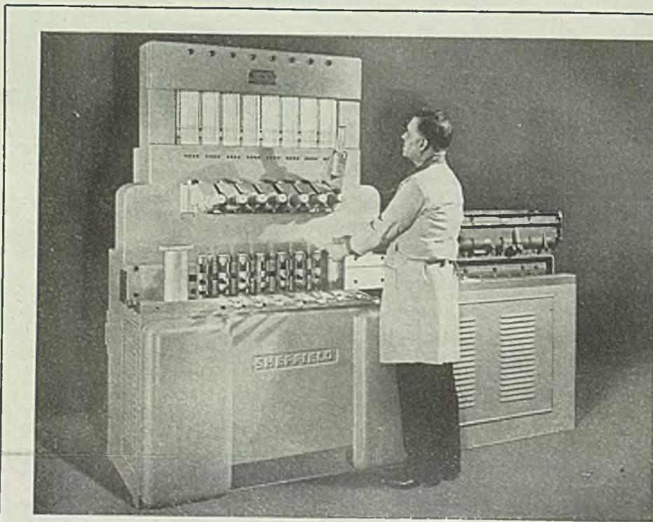
INSPECTING ENGINE BLOCKS: Gaging bore diameters of automobile cylinder blocks at 32 points for go and no go in less than one minute, this multiple spindle Precisionaire, developed by Sheffield Corp., Dayton, O., is an integral part of production line at Buick division of General Motors Corp. Instrument, weighing several thousand pounds, checks for diameter, taper and out-of-roundness of eight cylinder bores at four different points in each cylinder, and classifies them to an accuracy of 0.0003-in.
