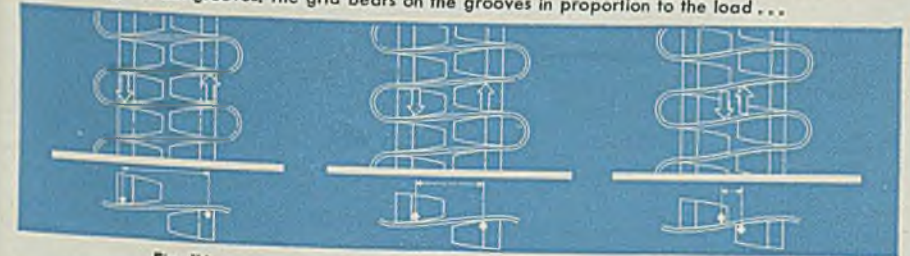
Fig. IV. Under light loads, the grid bears only at the outer edges of the grooves. This permits a long, free, elastic span between the outer edges of both hubs. Power is transmitted through almost the entire length of the grid rung... Fig. V. Under normal loads, the grid bears on a larger area of the grid grooves and the span of the grid run is shortened. It transmits more power and maintains its capacity to absorb shocks and dampen vibration... Fig. VI. Under peak loads, the grid rungs bear over almost all of the curved surfaces of the grooves. The span of the grid rung becomes very short. Under the impact of shock loads the grid flexes and continues to transmit power smoothly.
