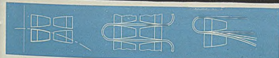
Fig. I. Grooves, in a precise arc, and with a radius and length proportional to the capacity of the coupling, are cut into two identical hubs of moderately high carbon steel—forged of Falk alloy cast steel... Fig. II. These grooves provide a slot for a grid member made of chrome alloy steel with an elastic limit of 180,000 pounds per square inch and an ultimate strength of 220,000 pounds per square inch... Fig. III. This grid fits snugly into the curved grooves cut into the hubs of the coupling. The grooves provide a scientifically cut bearing surface for the grid. This bearing surface extends from the outer to the inner edge of the grooves. The grid bears on the grooves in proportion to the load...
