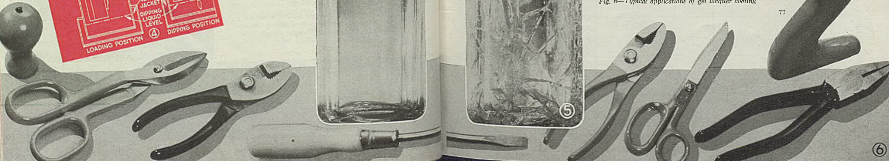
Fig. 6—Typical applications of gel lacquer coating
