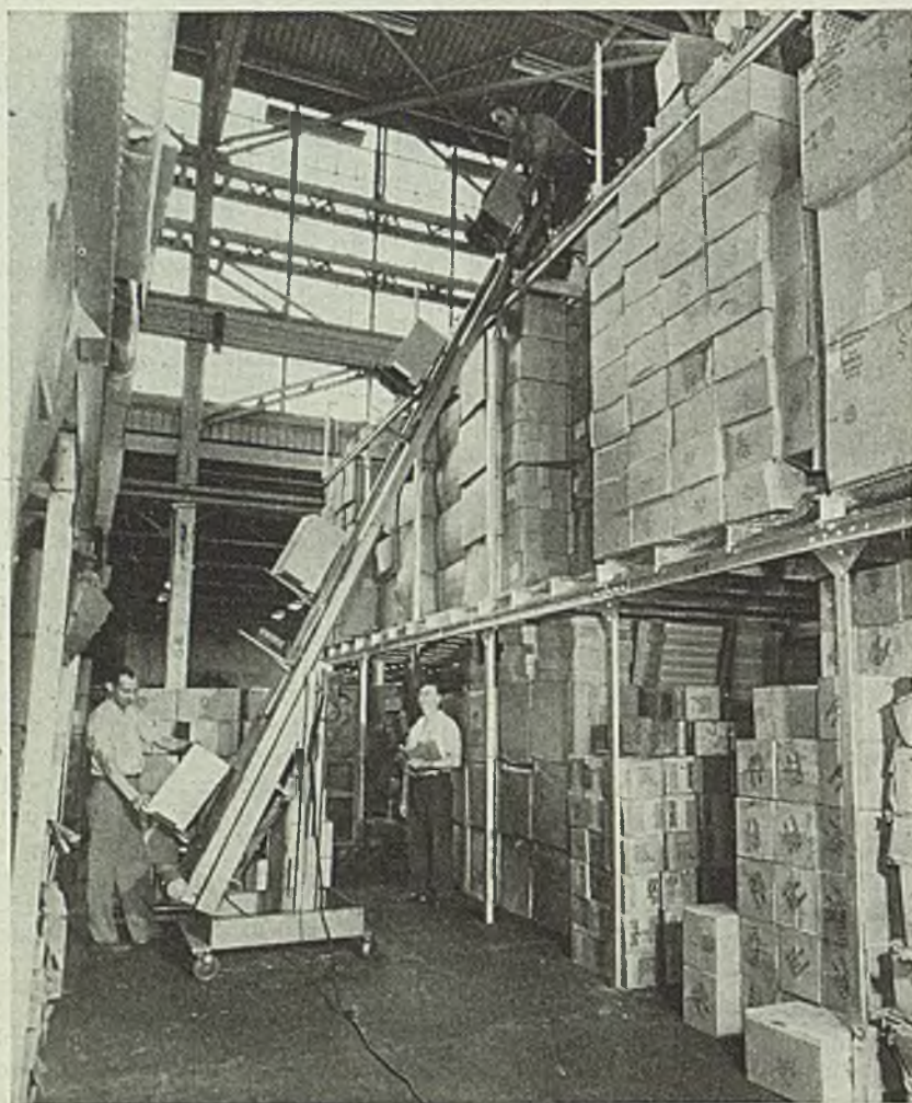
PACKAGE PILER: Spare parts are lifted automatically to storage racks at Buick's new parts warehouse at Grand Blanc, Mich. The new structure is 1200 feet long, contains more than 500,000 sq ft of floor space
