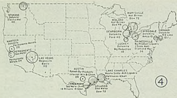
Fig. 4—Distribution of magnesium reduction plants. Shaded circles indicate ownership by DPC; white circles, private ownership. Operators are given in small letters. Numbers show capacities in millions of pounds per year
