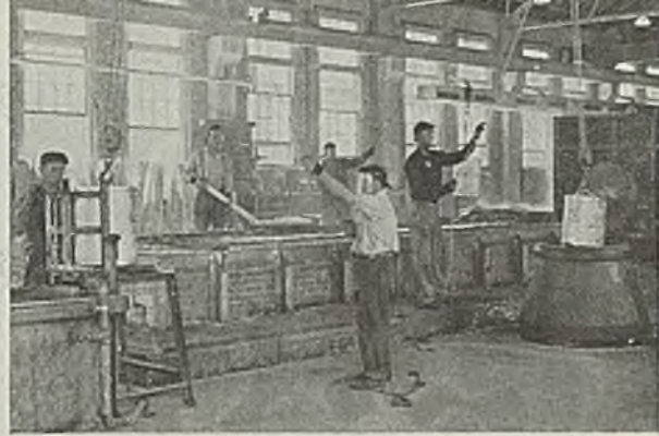
Fig. 33 (right)—Galvanizing kettle served by centrifuge when working on small parts
