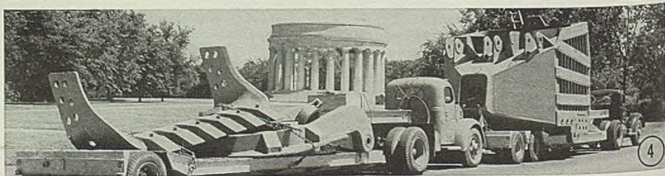
Fig. 4—Units of the big dipper on trucks enroute for assembly on the job
