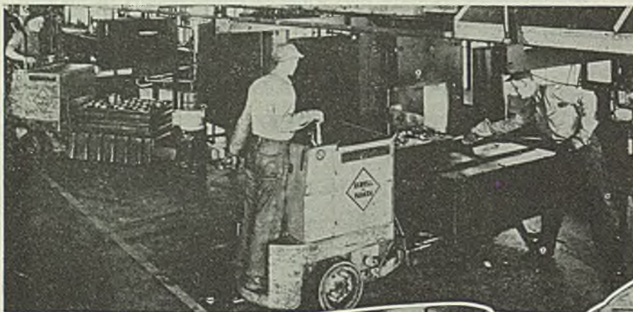
Fig. 1 (above) — Fabrication of quenching tanks for use with industrial power trucks, such as shown here, enabled one company to provide a continuous flow of parts from its heat treating department. Parts are raked from furnaces into tanks, moved to a cool location by trucks
