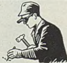
Hinged portion raised for chipping, grinding, peening or other eye hazardous work.
