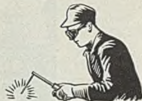
Willson-Weld* lenses down in correct position for welding.
