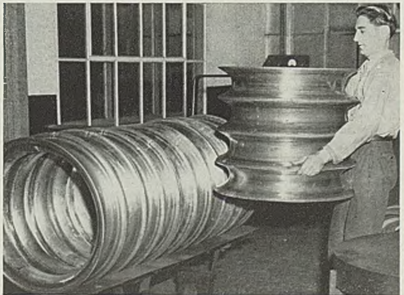
NO "TIRING" WORK: A 60 per cent saving in weight is achieved in these 28 aluminum truck tire flap curing rims fabricated by American Welding & Mfg. Co., Warren, O. Rims are rolled from \frac{3}{8} -in. flat strip and flash butt resistance welded
