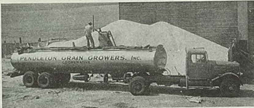
OREGON GRAIN CARRIER: Tractor truck with special tank trailer is being used by Pendleton Grain Growers Inc., Pendleton, Oreg., to move great quantities of grain to shipping points. The tractor truck is a recently announced model made at International Harvester Co.'s new Emeryville Works, Emeryville, Calif. It is estimated that the tank truck will have transported one-half million bushels of wheat by the end of 1946
