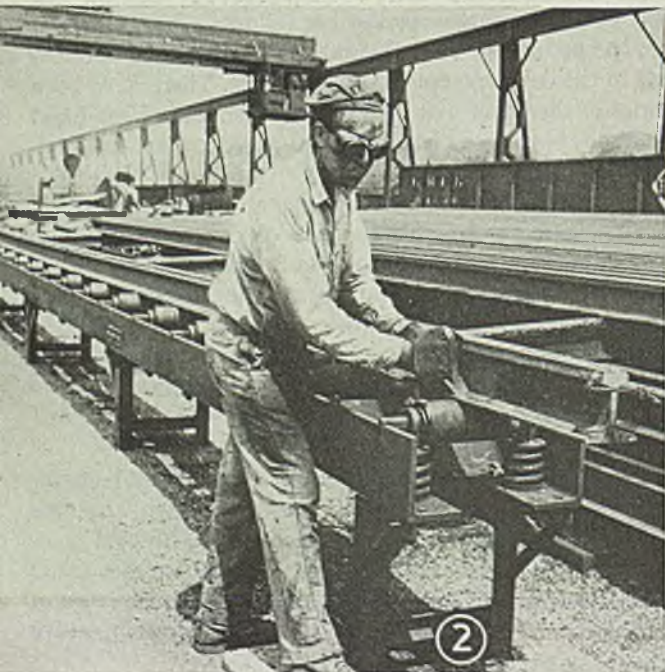
Fig. 3—First job in scrap handling is segregation. In-bound scrap (rear left) is sorted and loaded into out-bound cars (right), or palletized for shipment to stores and repair shops
