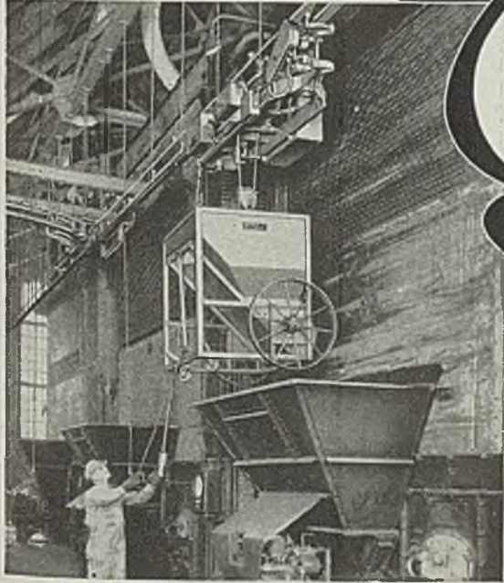
Buckets are rolled under discharge chutes of overhead bin or to outside coal storage and filled. They then are picked up and delivered to stoker hoppers by Tramrail System. Same equipment hauls ashes away.
