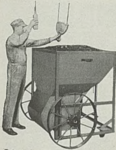
This bucket is \frac{3}{4} yard size and carries \frac{1}{2} ton of coal. It is used as shown below.
