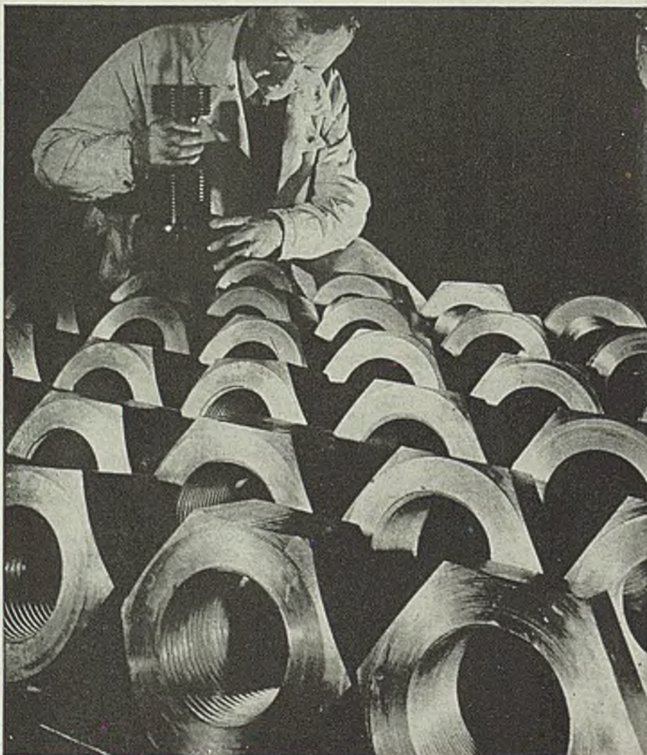
ACCURATE BEARING —RB&W Semi-finished Nuts have an accurate bearing surface at right angles to the axis of the thread. Special facing equipment and quality control insure satisfaction.
