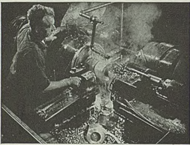
LARGEST NUTS —EMPIRE Nuts larger than 1½" bolt size are produced on machines of this type, especially adapted to RB&W requirements. Sizes up to 6½" across the flats are processed.
