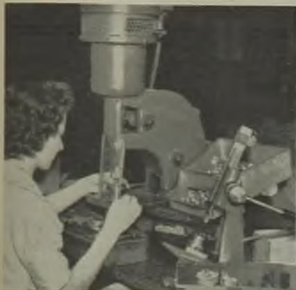
Assembly of "Bijou" rotor with oiled felt washers
