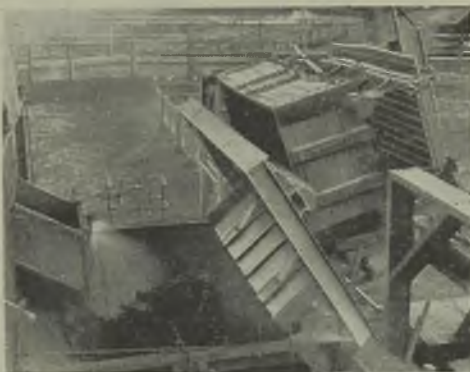
The green shale wagon tippler has a capacity of 230 tons per hour
