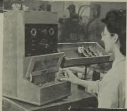
"Bijou" movements undergoing 2,000-V breakdown test and (right) a pneumatic machine for printing dials
