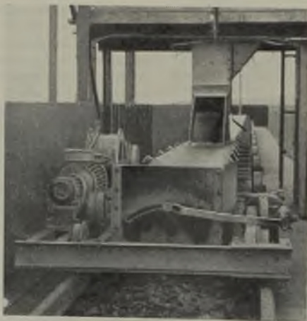
Endless reversible shuttle conveyor mounted on a travelling carriage
