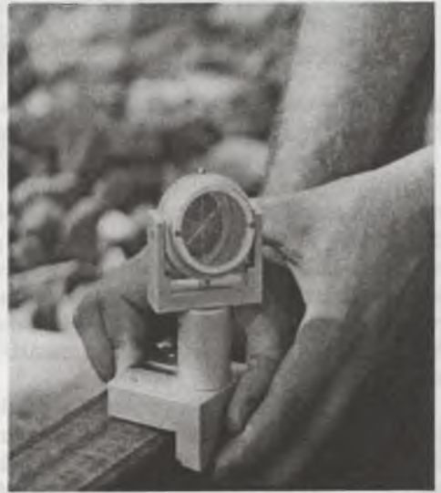
Rys.6. Lustro dalmiercze na szynie Fig.6. Range-finder glass prism on the rail
