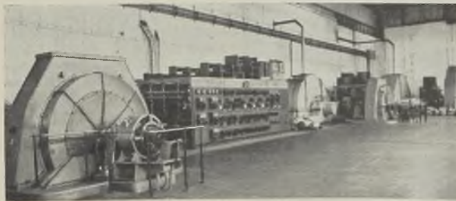
The first roughing stand is driven by a 2,500-H.P. slip-ring motor, and the second and third by 2,500-H.P. synchronous motors
