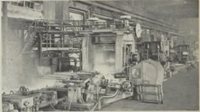
The three roughing stands of the hot strip mill
