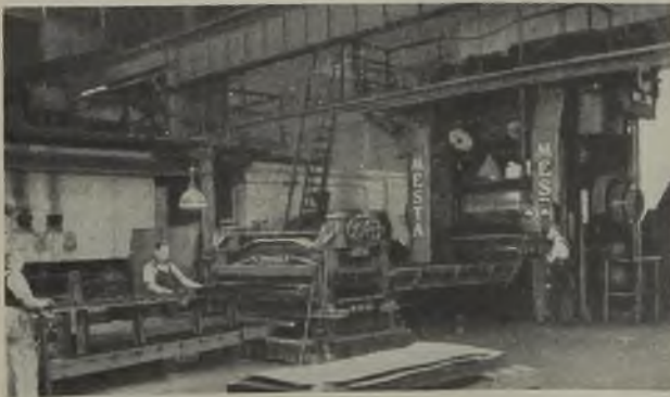
After annealing, the majority of the sheet steel is passed through "skin pass" mills for "temper" rolling
