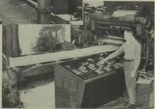
In the pickling lines (above) the scale on the strip is removed chemically. The strip is re-coiled in an up-coiler (right) at the delivery end of the pickling line
