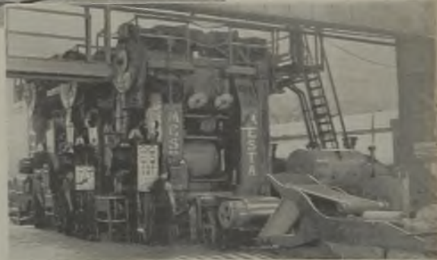
A winding reel at the delivery end of the mill has a specially controlled drive to ensure that the tightness of the coil remains constant
