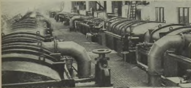
In the pickling lines (above) the scale on the strip is removed chemically. The strip is re-coiled in an up-coiler (right) at the delivery end of the pickling line
