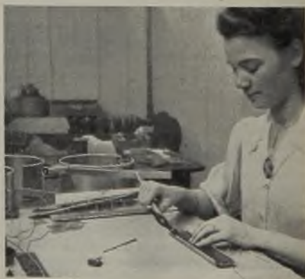
Finishing off "Genristo" band elements for plastic moulding work
