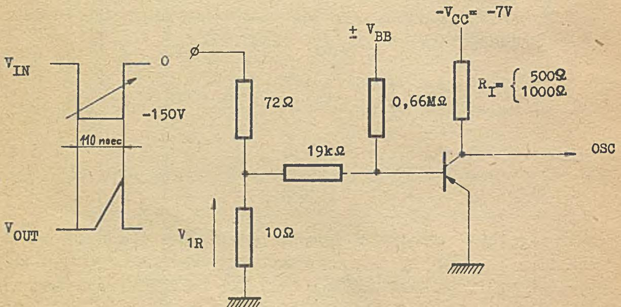
Fig. 5. Current drive measurements.
