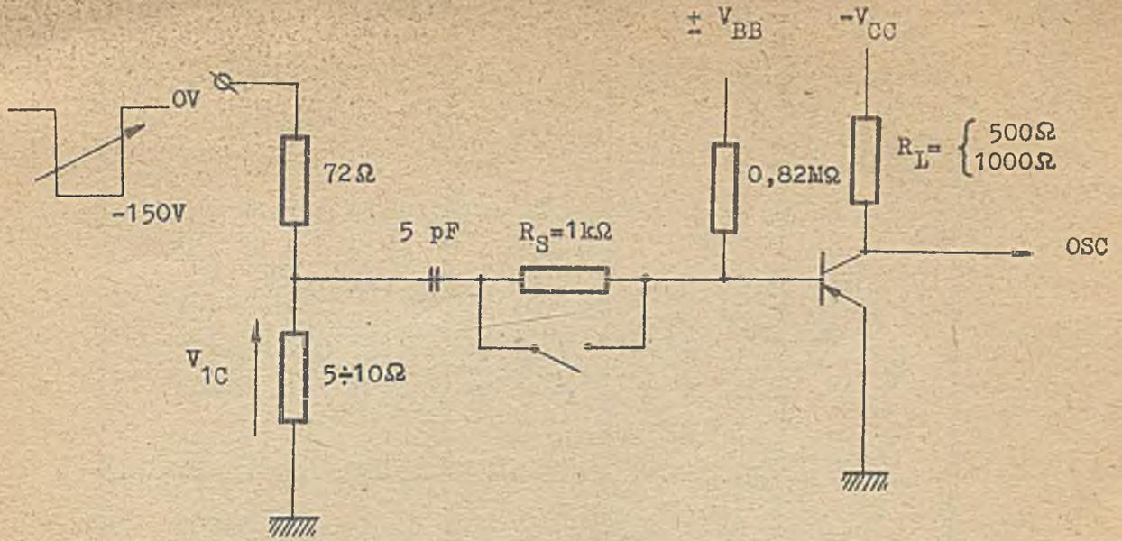
Fig. 3. The practical circuit for measurements of  $Q_E$ ,  $Q_B$ , and  $Q_V$ .
