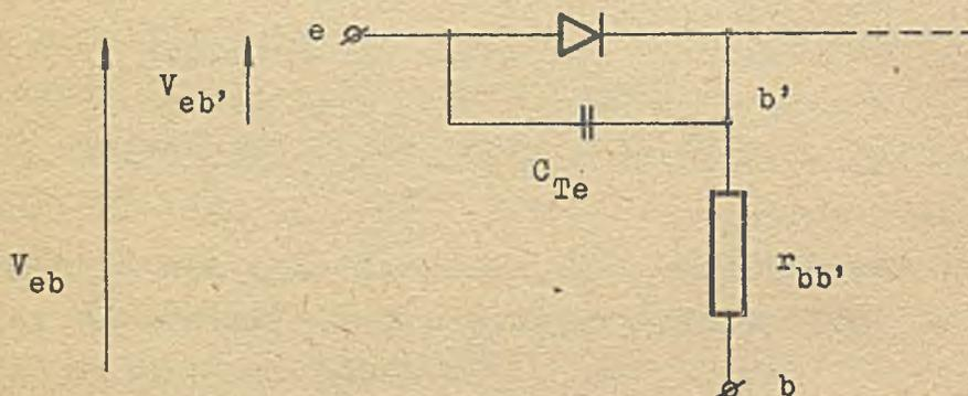
Fig. 1. Equivalent circuit for switching from the off state. The propagation phenomena are not yet taken into account.
