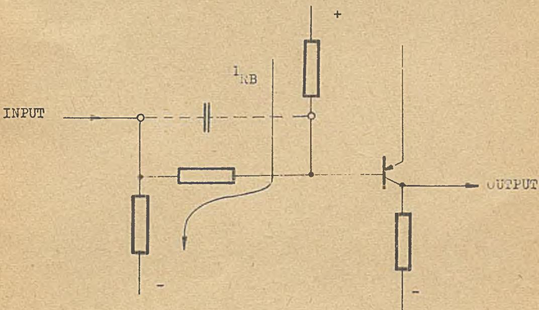
Fig. 11. The voltage-shifting principle.
