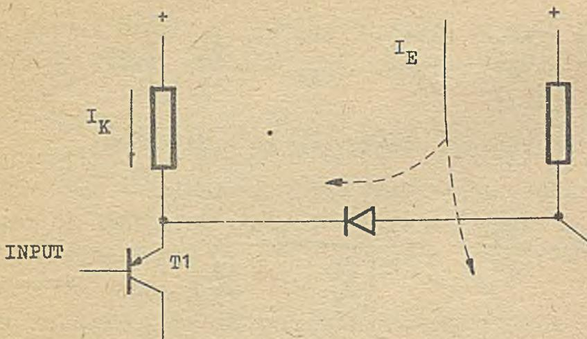
Fig. 9. Reduction of  $Q_E$  by means of the initial current  $I_K$ .
