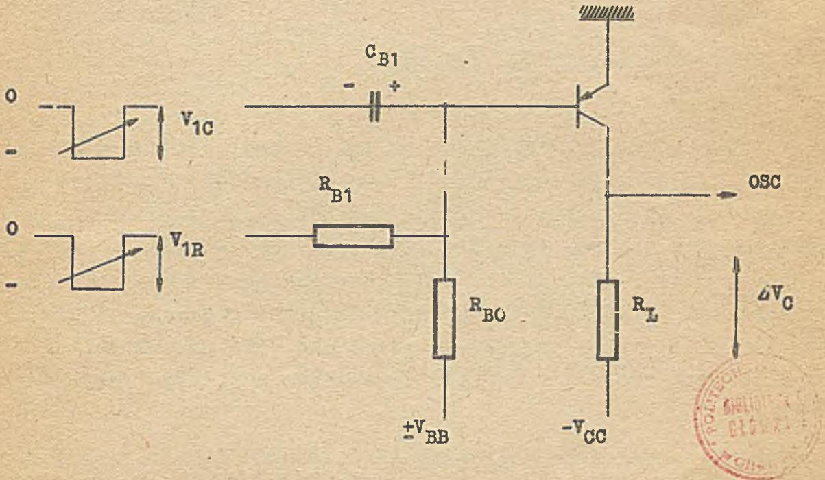
Fig. 2. The principle of measurement.
