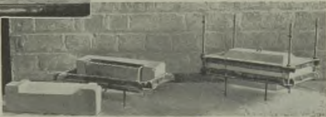
... Finally the bushing is placed in a framework of refractory bricks and the whole assembly, constituting the furnace, is held in a metal frame
