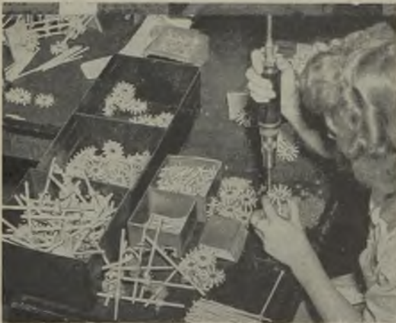
Assembling wafer type rotary switches
