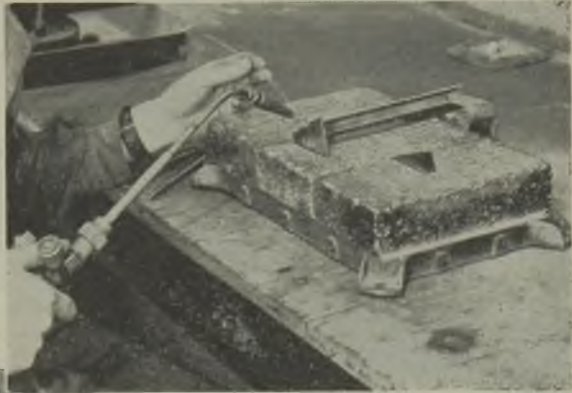
The nine pieces of the bushing are fused together . . .
