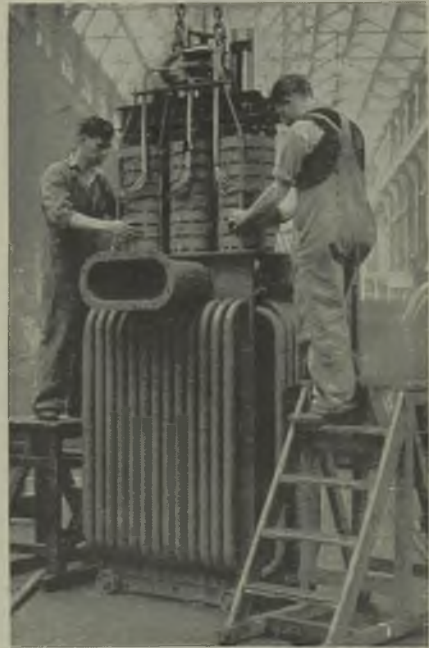
While still hot the internal unit is immersed in the oil-filled tank
