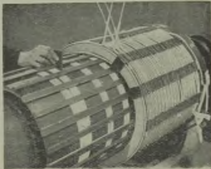
There comes a point where cross-over winding does not offer sufficient strength, and disc winding is then adopted
