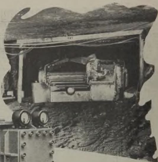
Battery-operated shuttle car at a charging station in a Scottish coal mine.
