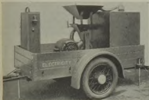
Nearly 150 "Essex" mills have been installed. Here is one mounted on a trailer for demonstration purposes
