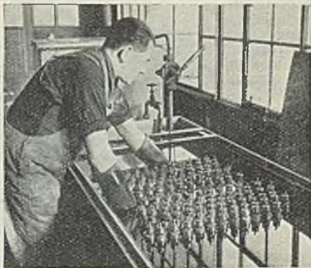
Armatures for Hoover vacuum cleaner motors being dipped in Bakelite varnish
