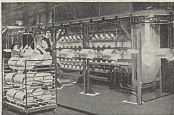
A Metrovick electric infra-red oven for paint stoving
