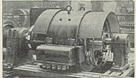
A 150 kW marine type d.c. generator for a floating dock. Disc lubrication is provided to meet tilting conditions
