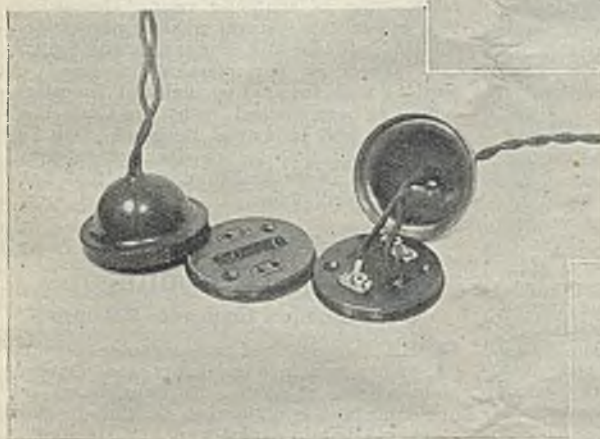
Fig. 5 (left). Electric ceiling rose, in two laminations of jute cloth, impregnated with pigment-filled phenolic resin.
