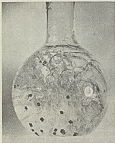
Fig 3. Effect of Microid flask-shaker† studied by ultra-high-speed camera. The circulation of the liquid is shown by the position of the blackened cubes of teak (of nearly the same density as water).
