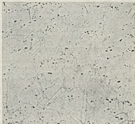
Fig. 8 (left). Micrograph of cast "tough pitch" copper, showing the eutectic of \text{Cu-Cu}_2\text{O} at grain boundaries. Fig. 9 (right). The same copper after working and annealing, showing a twinned crystal structure with globules of \text{Cu}_2 (both \times 100 ):
