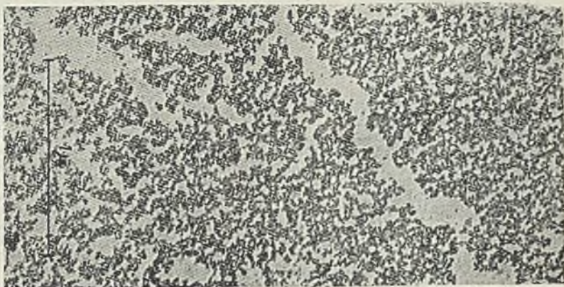
Fig. 3. Mercurochrome, in which most of the particles are of the order of .01 micron in diameter.
