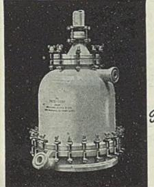
The Pneu-Pump is a compressed-air operated pump embodying in its design new principles. It has no moving mechanism. It is unchokable and operates from a very small supply of compressed air. The special model illustrated on the left is in chemical stoneware for pumping corrosive liquids. The separate parts are fastened with external clamps and cannot come into contact with the liquid being pumped. Write for particulars to the makers.
