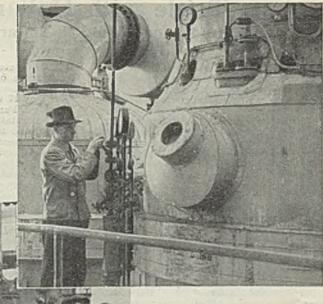
Fig. 2 (left). Splitting the soap by means of sulphuric acid which passes through the glass tubes illustrated.
