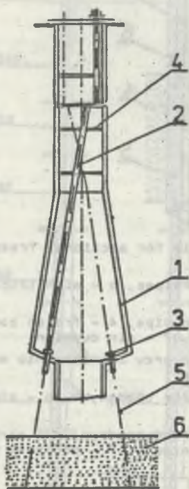
Fig. 4. The system of drilling freezing boreholes from the shaft: sectional freezing of "Tusanj" shaft in Yugoslavia
