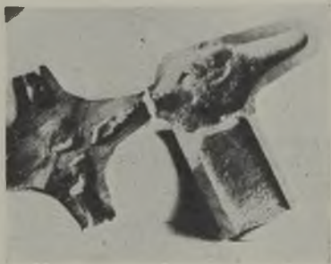
FIG. 9.—DEFECT CAUSED BY EXCESSIVE GAS GENERATION.
