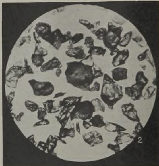
FIG. 2.—THE TYPE OF ANGULAR GRAIN USED.
