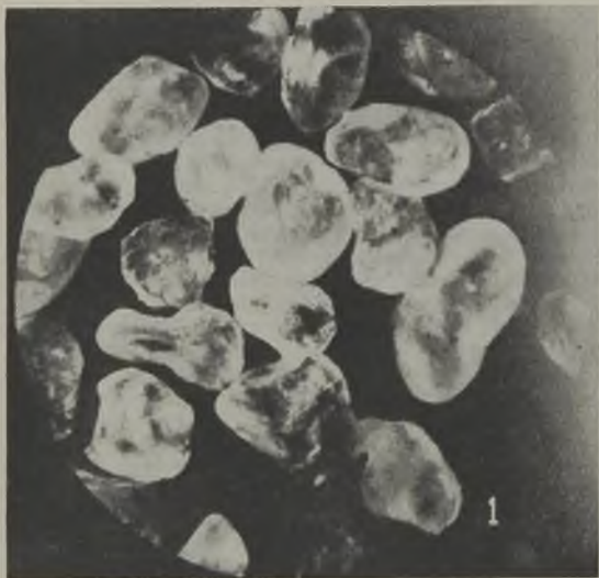
FIG. 1.—THE TYPE OF ROUNDED GRAIN SAND USED.
