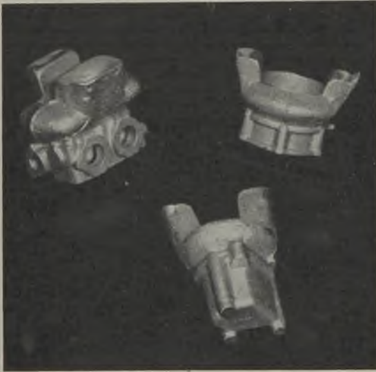
FIG. 6.—TYPICAL CASTINGS MADE FROM GRAVITY DIES TILTED DURING POURING.
