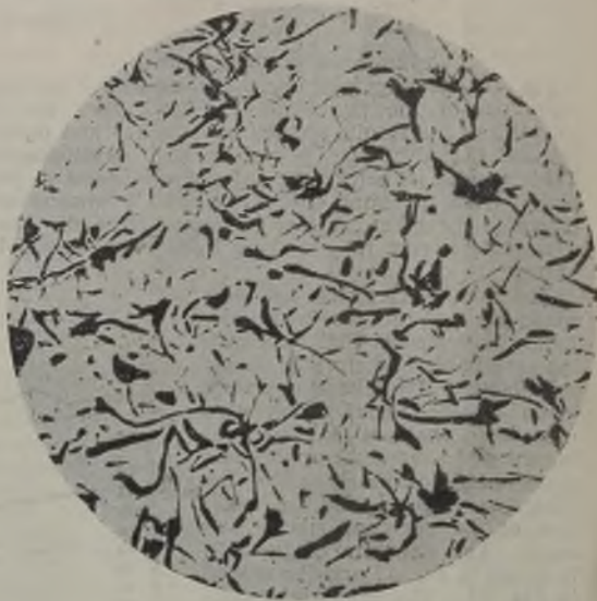
FIG. 12.—INOCULATED IRON FIRST TEST \times 75 .
