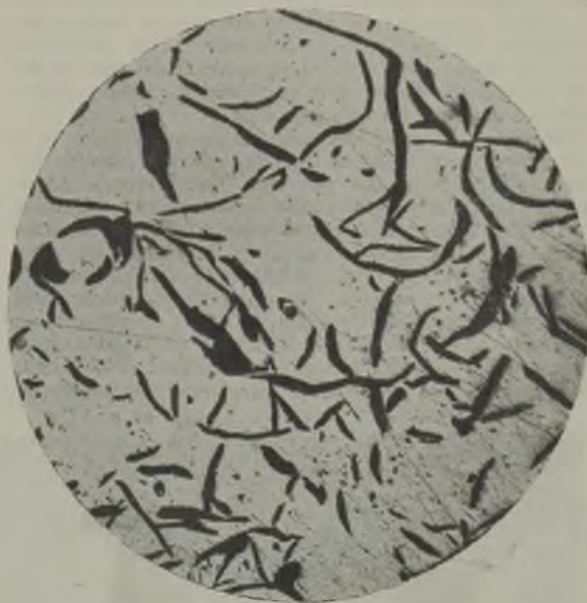
FIG. 16.—INOCULATED IRON CENTRE OF 5 IN. SECTION × 75.
