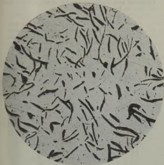
FIG. 15.—INOCULATED IRON EDGE OF 5 IN. SECTION × 75.
