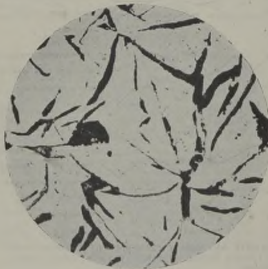
FIG. 13.—ORDINARY IRON CENTRE OF 5 IN. SECTION \times 75 .
