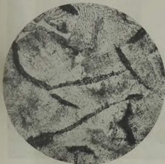
FIG. 17.—INOCULATED IRON EDGE OF 5 IN. SECTION ETCHED × 350.
