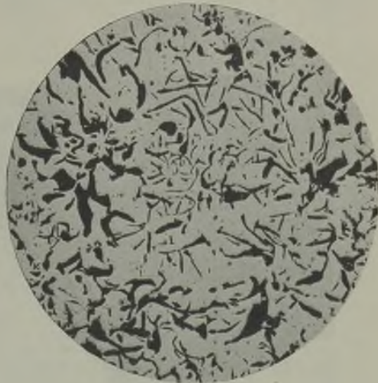
FIG. 22.—INOCULATED IRON CAST 15 MINS. AFTER FERRO-SILICON ADDITION \times 75 .
