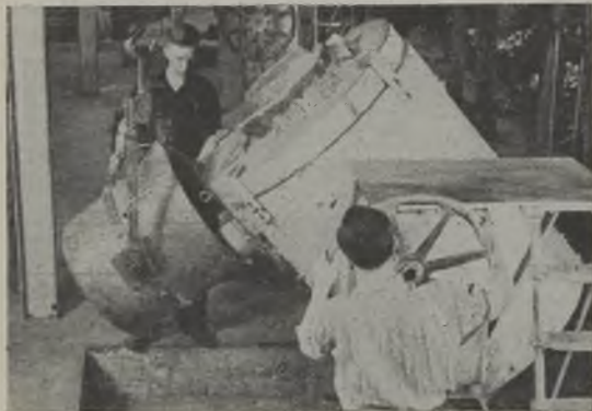
FIG. 28.—MOLTEN ALUMINIUM BEING Poured FROM MELTING FURNACE INTO GANISTER-LINED LADLE FOR TRANSFERRING TO MAINTAINING FURNACES.
