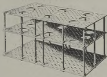
Set of finished nitriding trays cast in Brockhouse Heat-resisting Steel to operate at temperatures between 500° C. - 600° C. in ammonia fumes.
