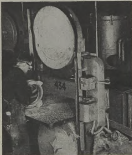
FIG. 36.—RISER OF "DIFFUSER VANE RING" CASTING BEING CUT OFF ON A "MIDSAW" 4-SPEED 30 IN. DIA. BANDSAW.
