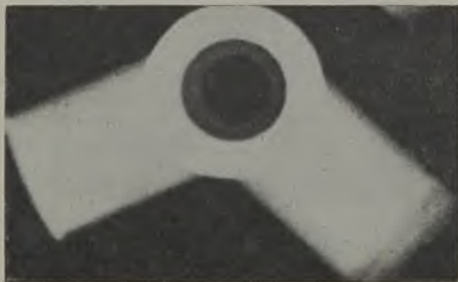
FIG. 22.—RADIOGRAPH OF SOUND CASTING OF SPRAY NOZZLE BODY.
