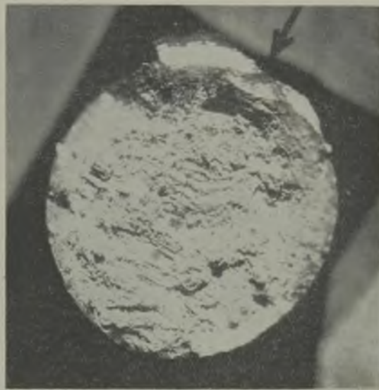
FIG. 6.—ABNORMAL TENSILE FRACTURE SHOWING INTERLOCKING OPPOSED DENDRITES. \times 4.5 .
