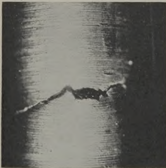
FIG. 7.—TENSILE FRACTURE CF. FIG. 6. LOCAL ZONE OF LOW ELONGATION AT DENDRITE JUNCTION. \times 4.5 .
