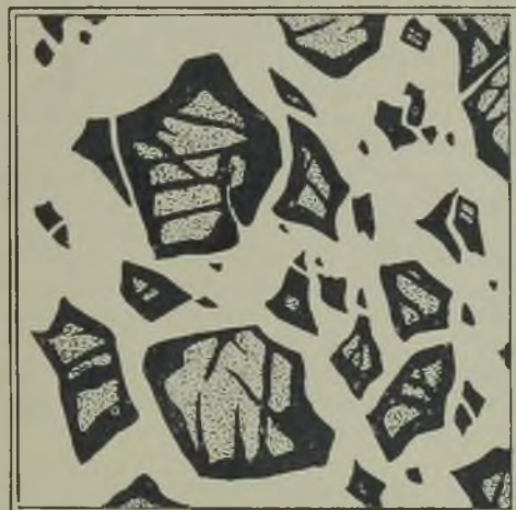
FIG. 5.—CHROMITE CRYSTALS IN MICRO-SECTION.
