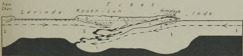
FIG. 3.—SECTION ACROSS INDIA AND CENTRAL ASIA TO ILLUSTRATE THE HYPOTHETICAL UNDERTHRUSTING OF ASIA, 2, BY GONDWANALAND, 1. Horizontal scale, 1:14,000,000. Vertical scale greatly exaggerated. Black represents sima supporting the sial (white) of the continental blocks. The dotted portion indicates the accumulated sediments of the Tethys which formerly lay between Gondwanaland and Asia. From Emile Argand (18, p. 349).
