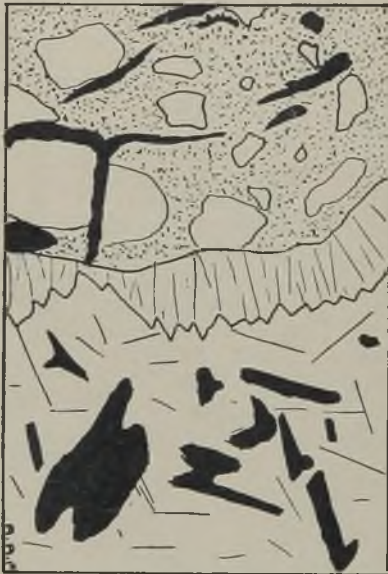
FIG. 4.—SHOWING COMPOSITE BRECCIA-FRAGMENT ENCRUSTED WITH QUARTZ CRYSTALS, AND FLOATING IN CALCITE CARRYING EUHEDRAL CHALCOHITE CRYSTALS (BLACK).
