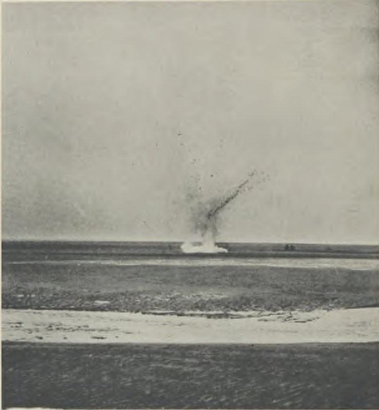
FIG. 8.—EXPLOSION OF EIGHT STICKS OF ARCTIC GELIGNITE BURIED AT A DEPTH OF 2 FT.
