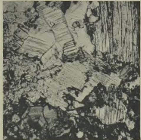
FIG. 7.—CASSITERITE, DARK-GREY WITH BLACK BORDER, AND MUSCOVITE, SHOWING MARKED CLEAVAGE, WITH QUARTZ IN VEINSTONE FROM PARC-AN-CHY MINE
